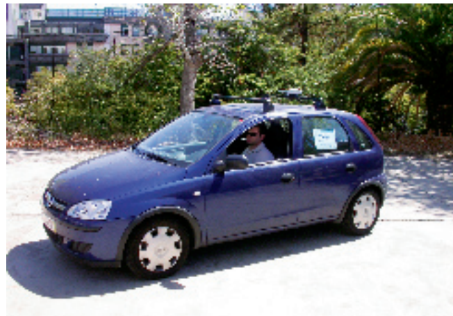
FIGURE 2 ARMAS test vehicle with GPS antenna visible on roof rack
